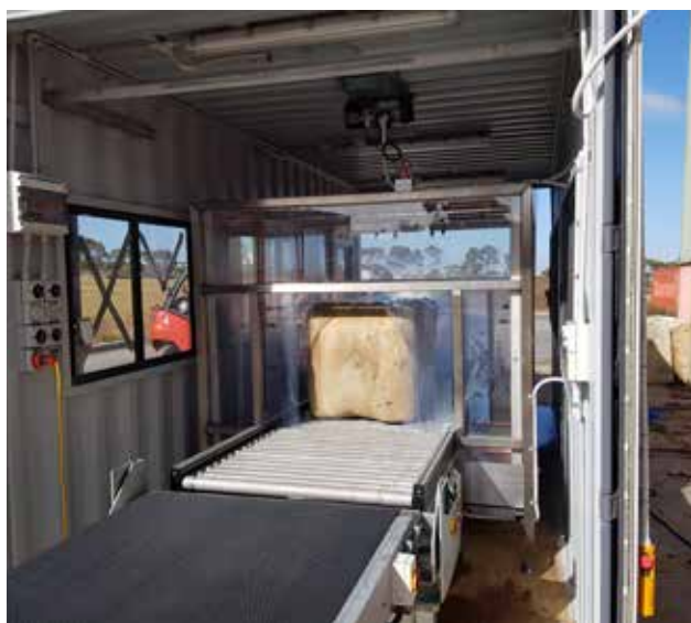
The wool bale sprayer in action during a field trial (Source: AWTA)
